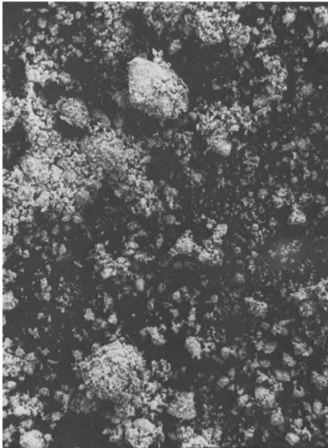
Fig. 2. \text{ZrO}_2 powders (3 mol% \text{Y}_2\text{O}_3 ). Bar = 100\ \mu\text{m} .
